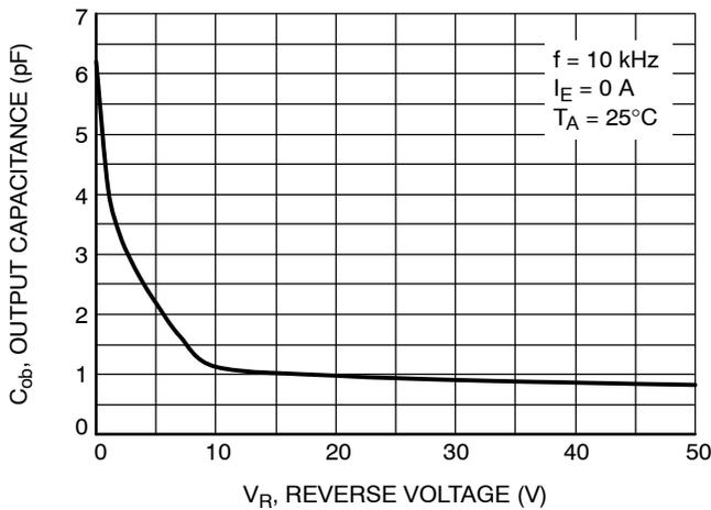
Figure 4. Output Capacitance
