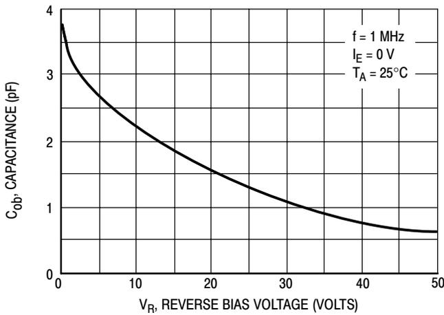
Figure 4. Output Capacitance
