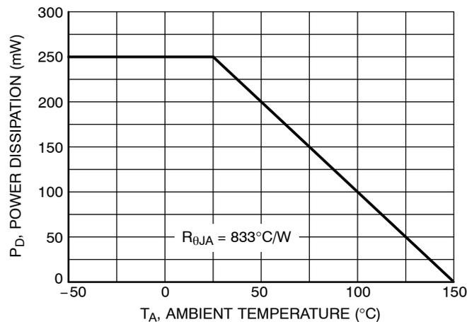
Figure 1. Derating Curve
