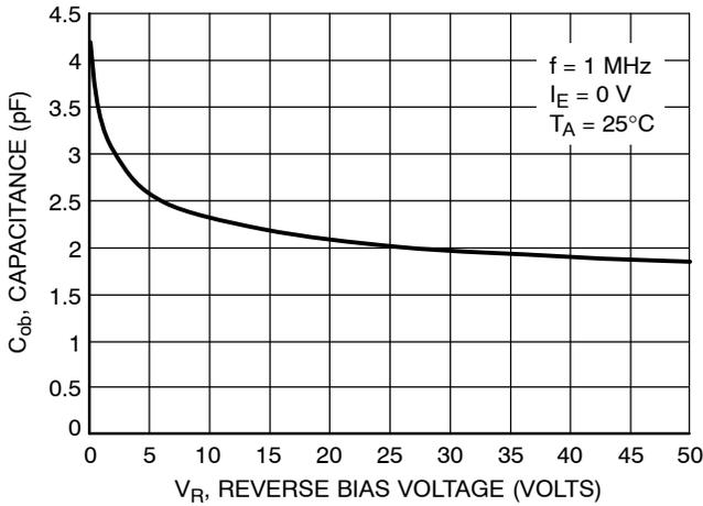
Figure 9. Output Capacitance
