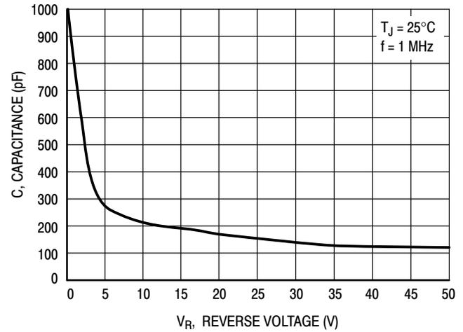
Figure 4. Typical Capacitance
