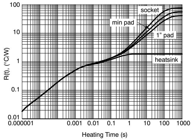
**Figure 7. Single-Pulse Transient Response Curves, Various Mounting Conditions**
