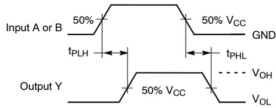
**Figure 3. Switching Waveforms**
