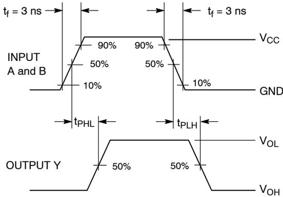
Figure 4. Switching Waveform
