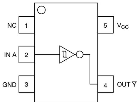
Figure 1. Pinout
