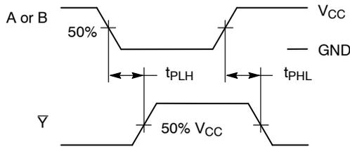
Figure 3. Switching Waveform
