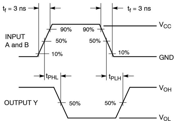
Figure 3. Switching Waveform
