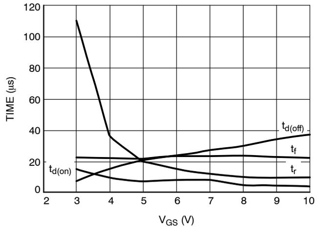
Figure 9. Resistive Switching
