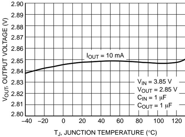
Figure 3. Output Voltage vs. Temperature –  $V_{OUT} = 2.85\text{ V}$
