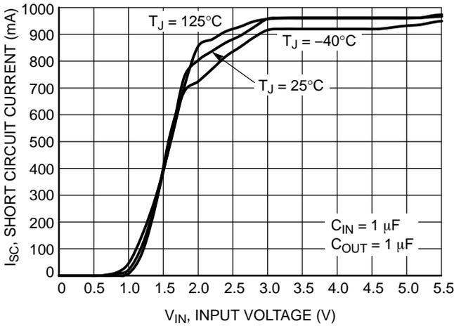
Figure 11. Short Circuit Current vs. Input Voltage
