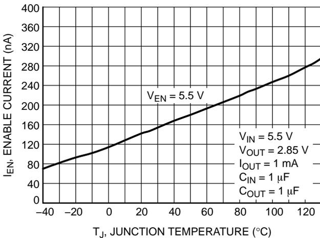
Figure 13. Current to Enable Pin vs. Temperature
