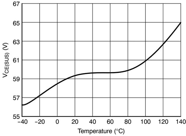
Figure 3. Typical  $V_{CE(SUS)}$
