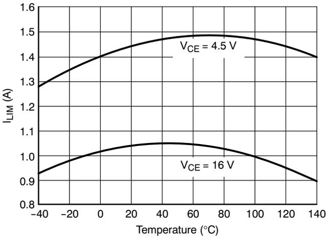
Figure 5. Typical Output Current Limit,  $V_{CC} = 5.0 V$
