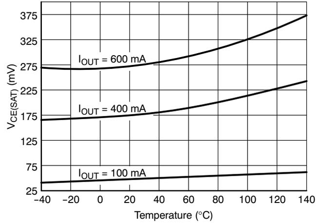
Figure 4. Typical Output On Voltage,  $V_{CC} = 4.0 V$
