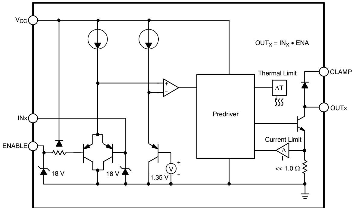
Figure 2. Simplified Block Diagram - Each Driver
