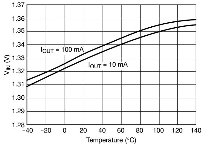
Figure 9. Typical Input Threshold Voltage, V<sub>CC</sub> = 5.0 V
