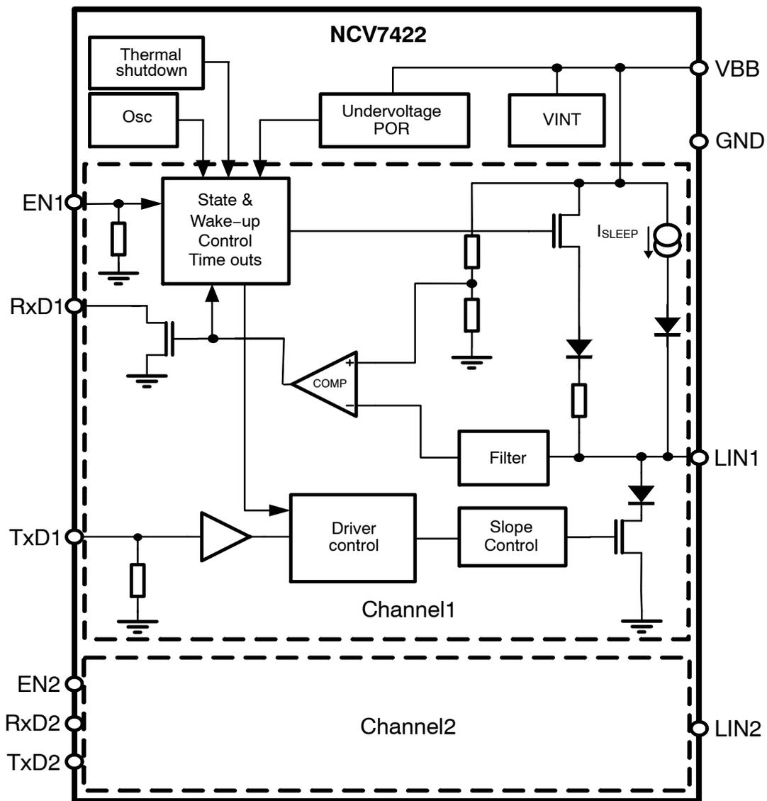
Figure 1. Block Diagram
