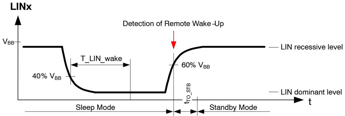
Figure 4. Remote (LIN) Wake-up Detection
