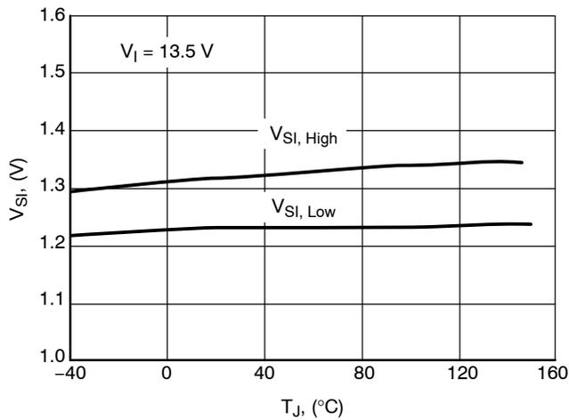
Figure 11. Sense Threshold  $V_{S1}$  vs. Temperature  $T_J$
