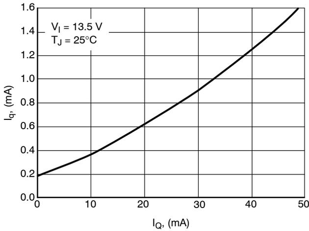
Figure 15. Current Consumption  $I_q$  vs. Output Current  $I_Q$
