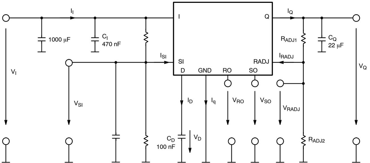
Figure 2. Measuring Circuit
