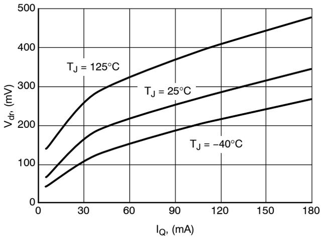
Figure 7. Drop Voltage  $V_{dr}$  vs. Output Current  $I_Q$
