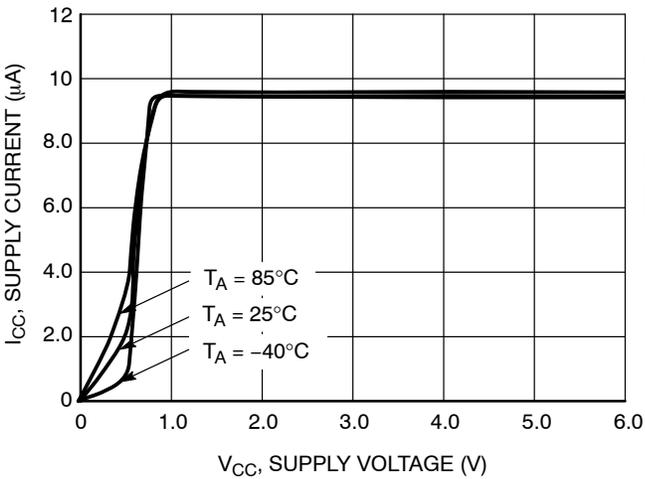
**Figure 3. NCS2220A Supply Current versus Supply Voltage/Comparator**
