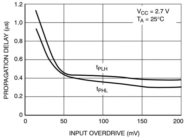
**Figure 10. NCS2220A Propagation Delay versus Input Overdrive**
