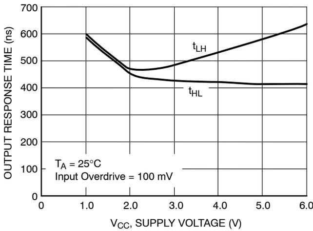
**Figure 9. NCS2220A Output Response Time versus Supply Voltage**
