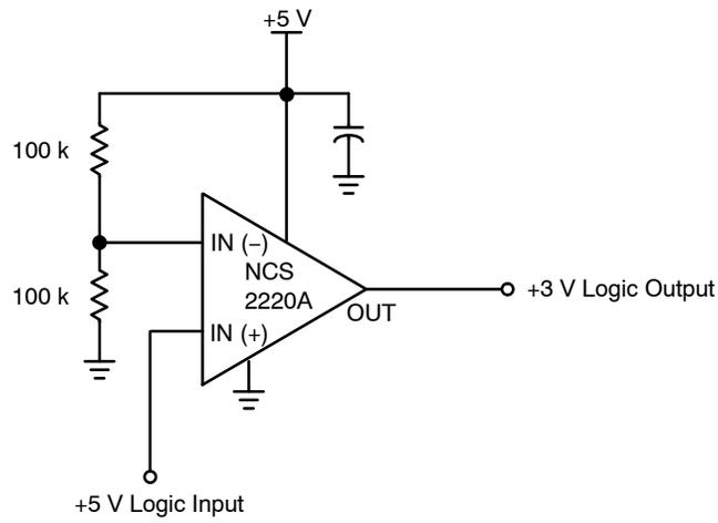
This circuit converts 5 V logic to 3 V logic. Using the NCS2220A allows for full 5 V logic swing without creating overvoltage on the 3 V logic input.
