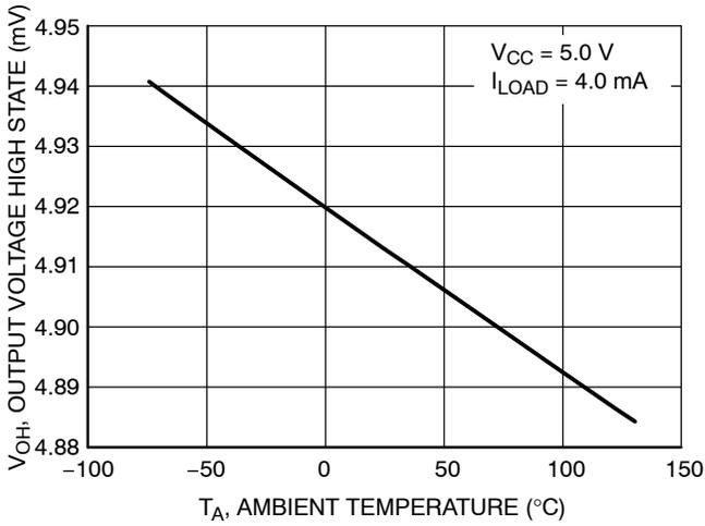
**Figure 7. NCS2220A Output Voltage High State versus Temperature**
