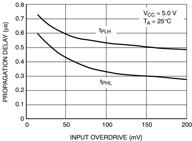
**Figure 11. NCS2220A Propagation Delay versus Input Overdrive**
