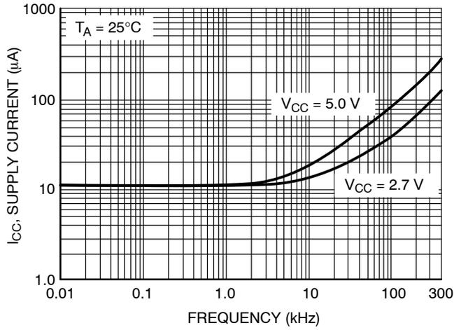
**Figure 2. NCS2220A Supply Current versus Output Transition Frequency/Comparator**
