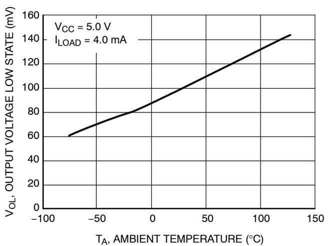
**Figure 6. NCS2220A Output Voltage Low State versus Temperature**
