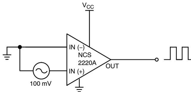
**Figure 18. Zero-Crossing Detector**
