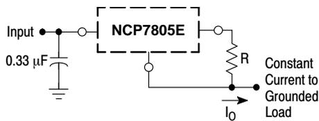
The NCP7800E regulators can also be used as a current source when connected as above. In order to minimize dissipation the NCP7805E is chosen in this application. Resistor R determines the current as follows:
