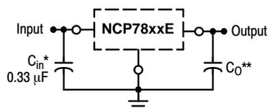
A common ground is required between the input and the output voltages. The input voltage must remain typically 2.0 V above the output voltage even during the low point on the input ripple voltage.
