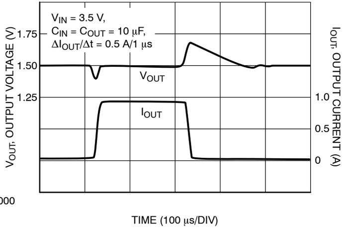
**Figure 22. Load Transient**
