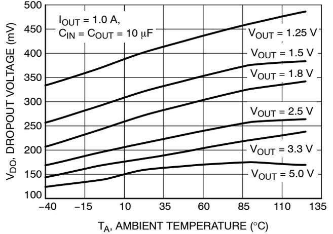
**Figure 16. Dropout Voltage vs. Temperature**
