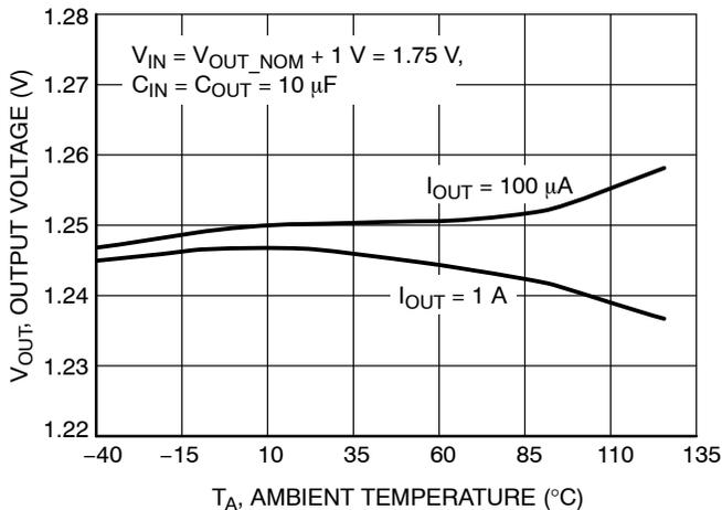
**Figure 11. Output Voltage vs. Temperature**
