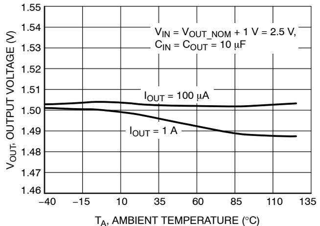
**Figure 12. Output Voltage vs. Temperature**
