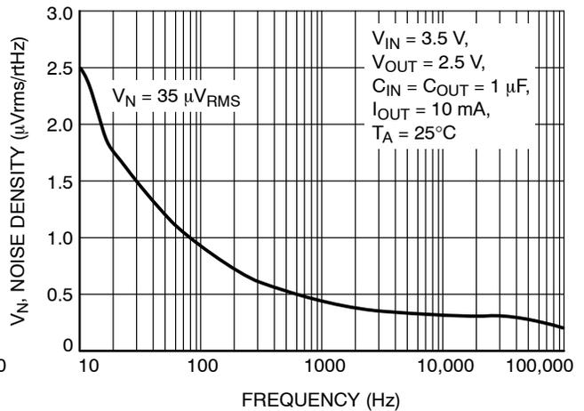
**Figure 20. Noise Density vs. Frequency**
