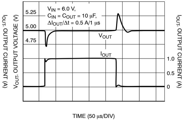
**Figure 24. Load Transient**
