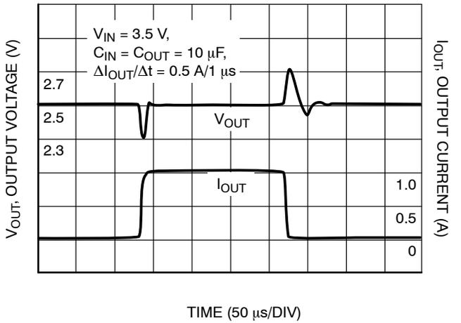
**Figure 23. Load Transient**
