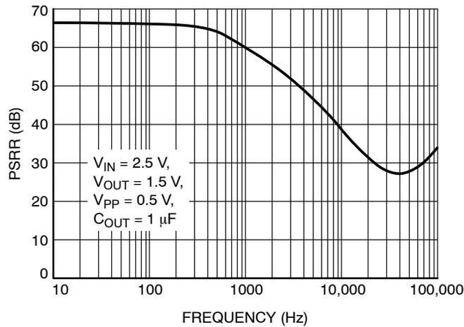
**Figure 31. PSRR vs. Frequency**
