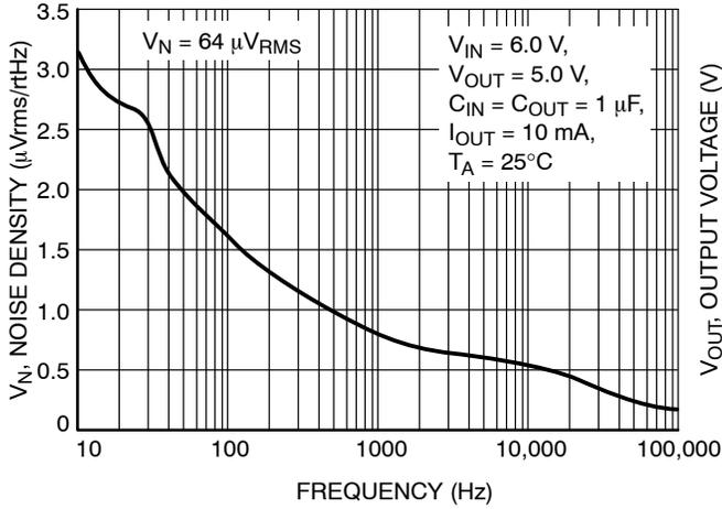
**Figure 21. Noise Density vs. Frequency**
