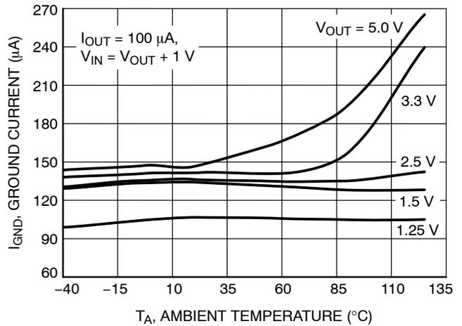
**Figure 18. Ground Current vs. Temperature**
