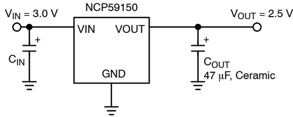
Figure 3. Fixed 2.5 Regulator in D<sup>2</sup>PAK-3 Package
