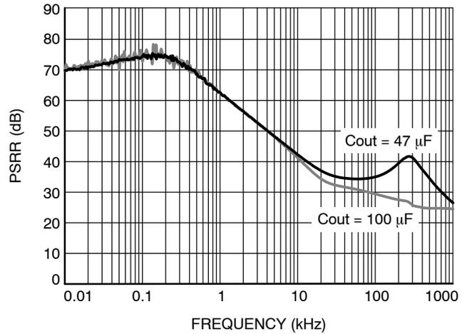
**Figure 17. PSRR vs. Frequency,  $V_{in} = 3.5\text{ V}$  + 200 mVpp Modulation,  $V_{out} = 2.5\text{ V}$ ,  $I_{out} = 0.5\text{ A}$**
