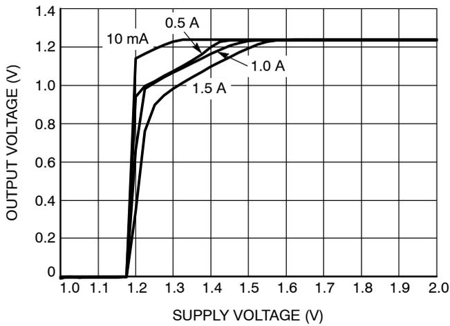
**Figure 6. Dropout Characteristics**
