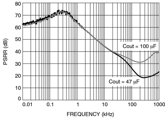
**Figure 18. PSRR vs. Frequency,  $V_{in} = 3.5\text{ V}$  + 200 mVpp Modulation,  $V_{out} = 2.5\text{ V}$ ,  $I_{out} = 1.5\text{ A}$**
