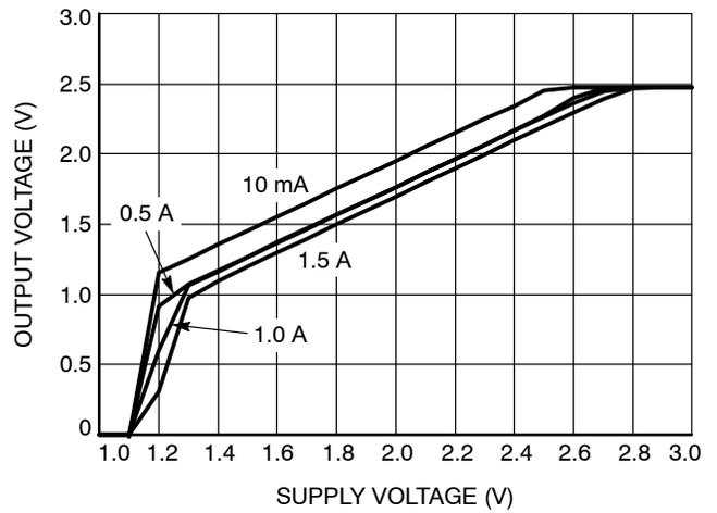
**Figure 7. Dropout Characteristics**
