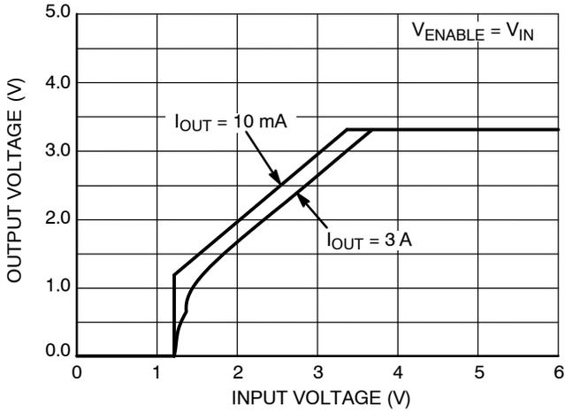
Figure 6. Dropout Characteristics
