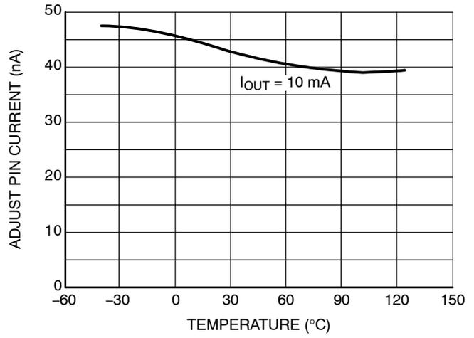
Figure 17. Adjust Pin Current vs. Temperature
