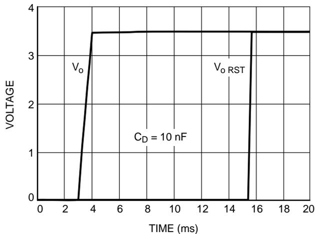
Figure 9.  $V_o$  and  $V_o RST$  versus Time
