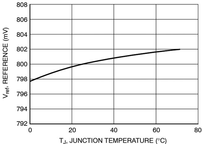
**Figure 4. Reference Voltage (V<sub>ref</sub>) vs. Temperature**
