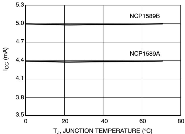
**Figure 5. I<sub>CC</sub> vs. Temperature**
