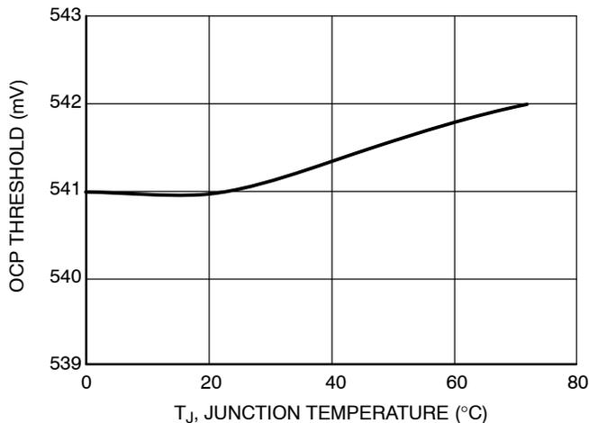
**Figure 6. OCP Threshold at 55k vs. Temperature**
