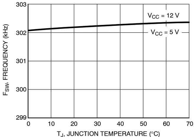
**Figure 3. Oscillator Frequency (F<sub>sw</sub>) vs. Temperature**
