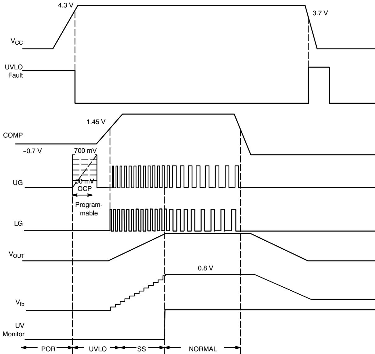
Figure 7. Typical Startup Sequence
