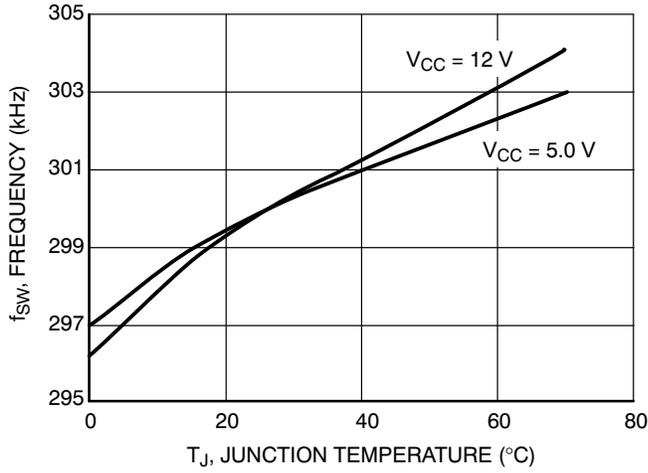
Figure 3. Oscillator Frequency ( $f_{sw}$ ) vs. Temperature
