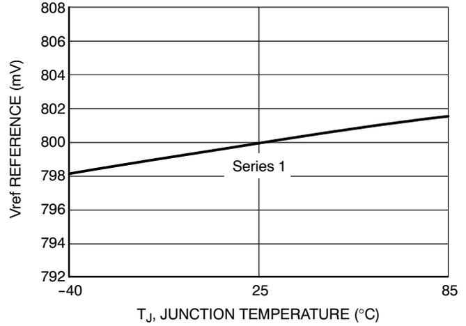
Figure 4. Reference Voltage ( $V_{ref}$ ) vs. Temperature
