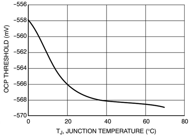
Figure 6. OCP Threshold with 55k Rset vs. Temperature
