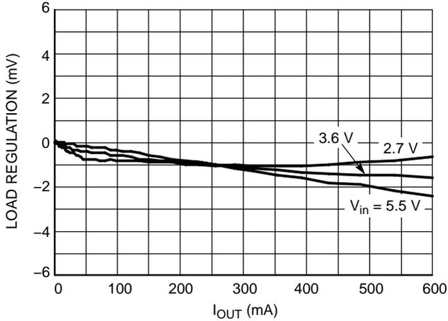
Figure 24. Load Regulation vs. Input Voltage
