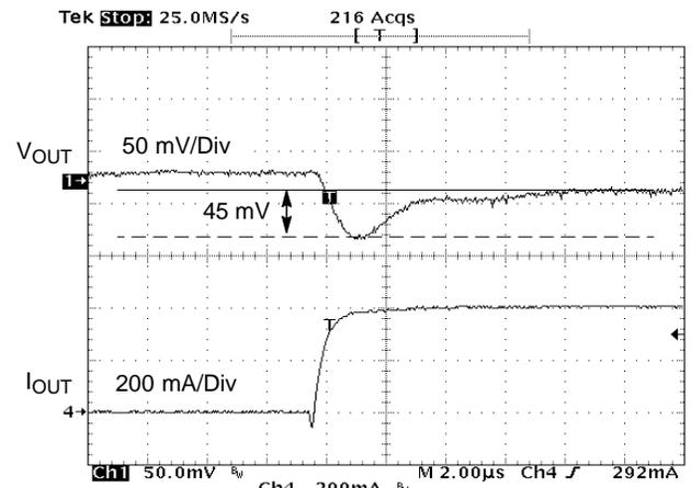
Figure 33. Load Transient Response
