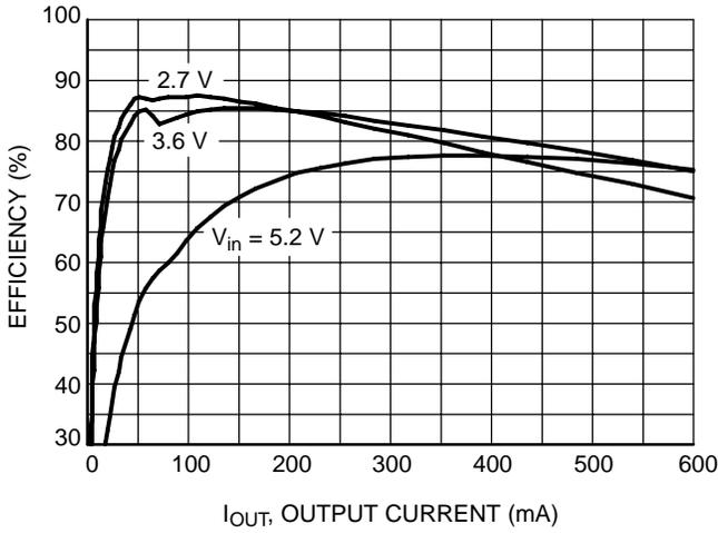
Figure 20. Efficiency vs. Output Current
