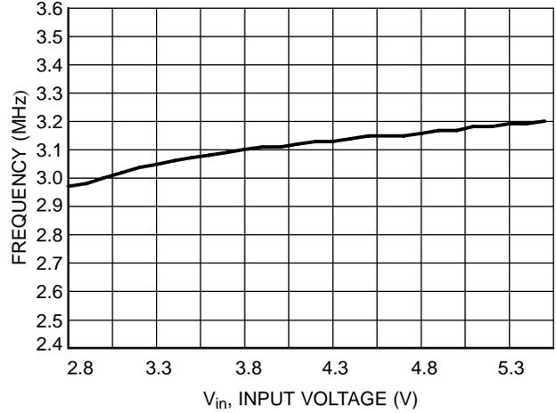
Figure 19. Switching Frequency vs. Input Voltage
