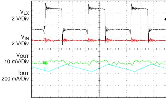
Figure 18. PWM Mode of Operation
