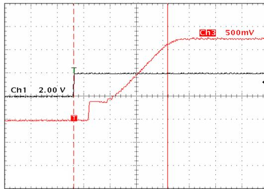
Figure 17. Soft Start Time ( $V_{IN} = 3.6 \text{ V}$ )
