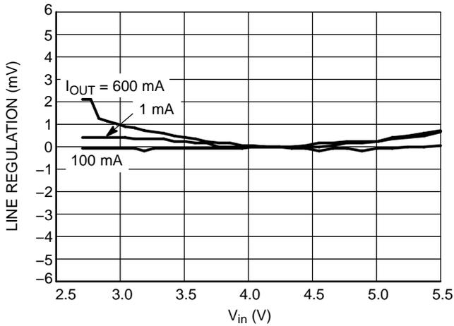
Figure 26. Line Regulation vs. Output Current
