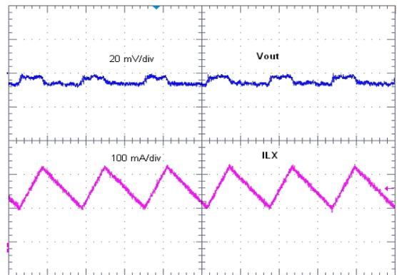
Figure 14. Step Down Converter PWM Mode Operation
