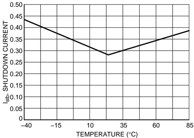
Figure 28. Shutdown Current vs. Temperature
