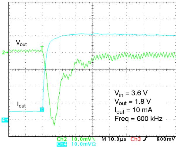
Figure 28. Load Transient from 10 to 100 mA
