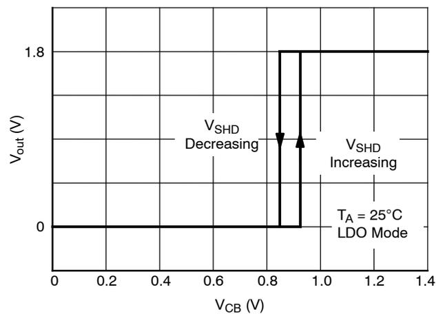
Figure 17. Output Voltage versus Shutdown Pin Voltage
