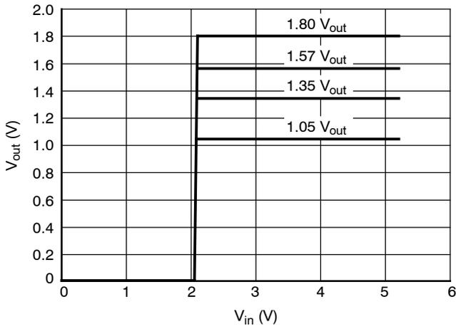
**Figure 18. Output Voltage versus PWM Input Voltage**
