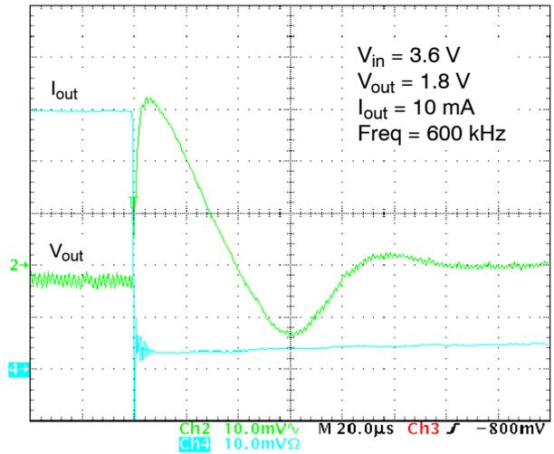
Figure 29. Load Transient from 100 to 10 mA
