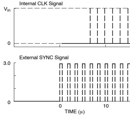
**Figure 6. Transition Waveforms from LDO to PWM Mode**
