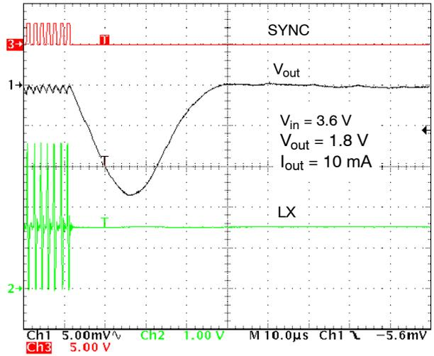
Figure 25. Transition from PWM to LDO Mode
