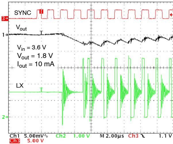
Figure 24. Transition from LDO to PWM Mode
