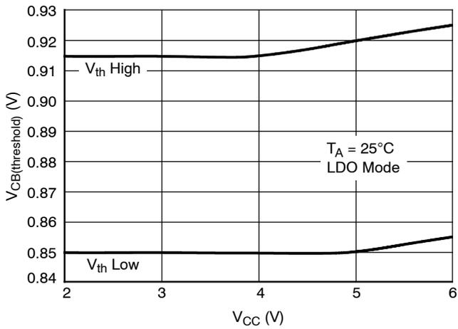
Figure 14. V<sub>CC</sub> Input Voltage versus CB Threshold
