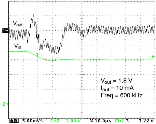
Figure 27. Line Transient from 3.6 to 3.0 V
