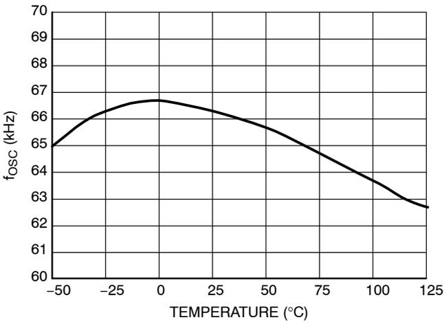
Figure 13. Oscillator Frequency  $f_{osc}$  for the 65 kHz version
