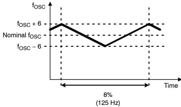
Figure 34. Frequency Jittering
