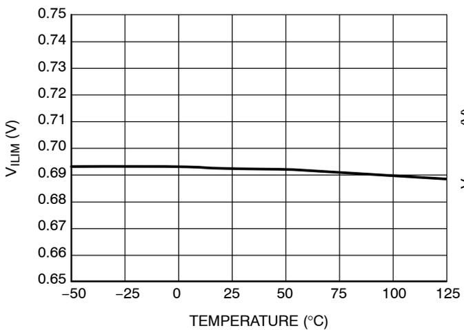
Figure 7. Maximum Internal Current Setpoint
