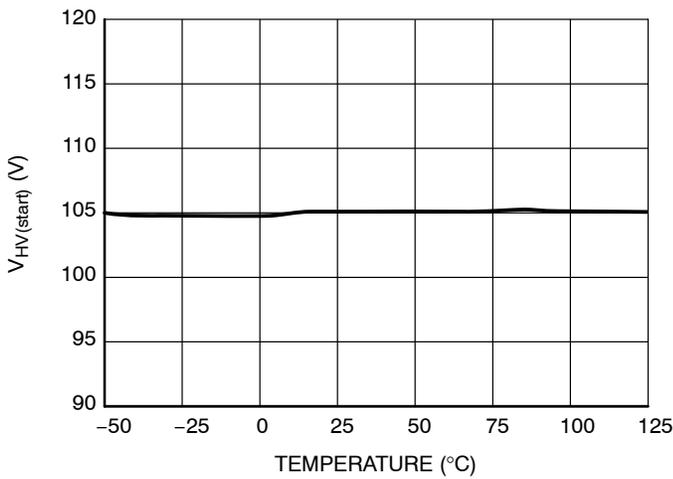
Figure 5. Brown-out Device Start Threshold
