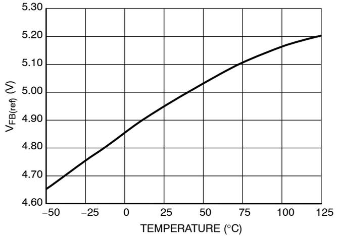
Figure 12. FB Pin Open Voltage  $V_{FB(ref)}$
