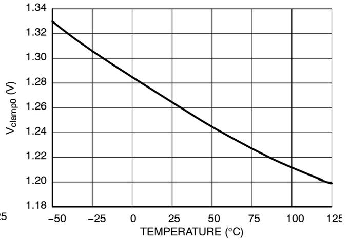
**Figure 26. Latch Pin Open Voltage  $V_{clamp0}$**
