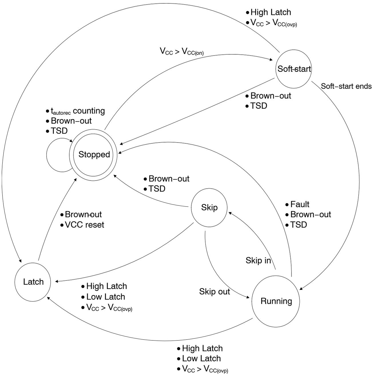
With Fault=  $\left( \begin{array}{l} \bullet t_{fault} \text{ expires} \\ \bullet V_{CS} > V_{CS(stop)} \\ \bullet V_{CC} < V_{CC(off)} \end{array} \right)$
