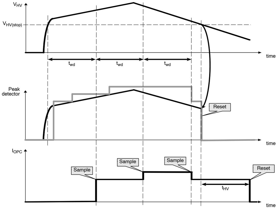
**Figure 42. Overpower Compensation**
