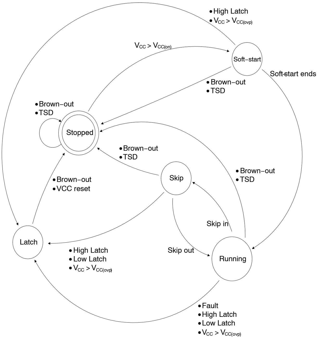
With Fault=  $\left( \begin{array}{l} \bullet t_{\text{fault}} \text{ expires} \\ \bullet V_{CS} > V_{CS(\text{stop})} \\ \bullet V_{CC} < V_{CC(\text{off})} \end{array} \right.$
