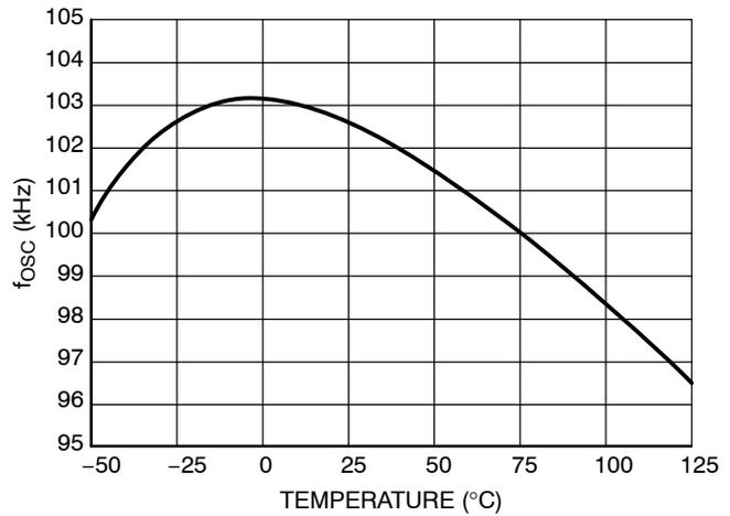
Figure 14. Oscillator Frequency  $f_{osc}$  for the 100 kHz version
