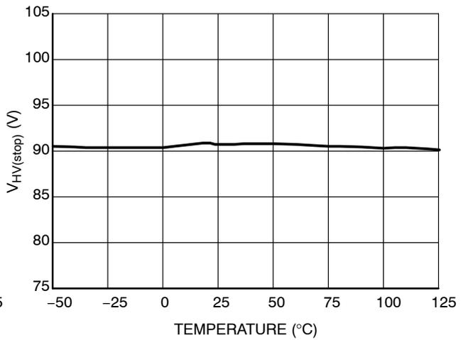
Figure 6. Brown-out Device Stop Threshold
