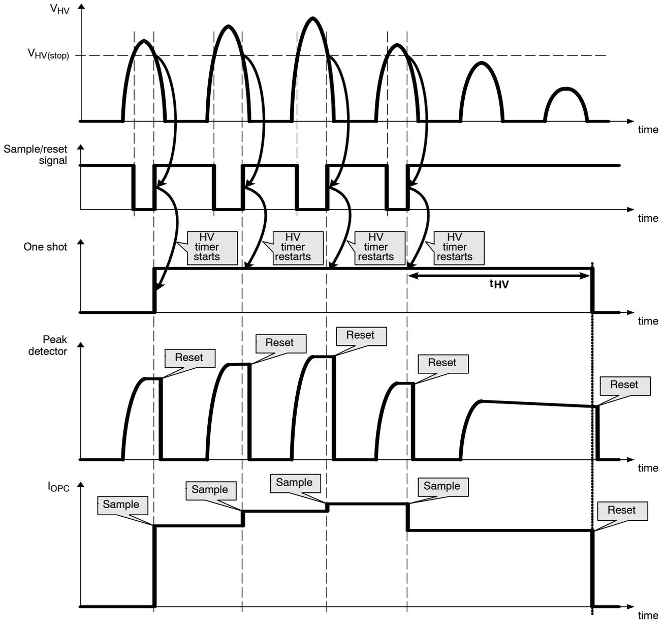
Figure 41. Overpower Compensation
