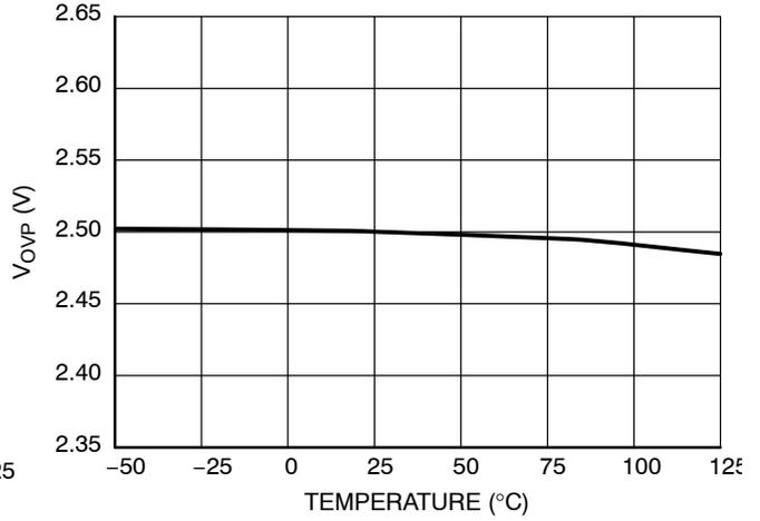
**Figure 24. Latch Pin High Threshold  $V_{OVP}$**
