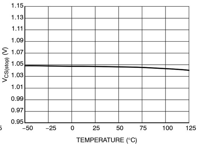
Figure 8. Threshold for Immediate Fault Protection Activation
