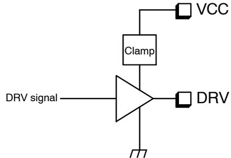
Figure 35. Clamped Driver
