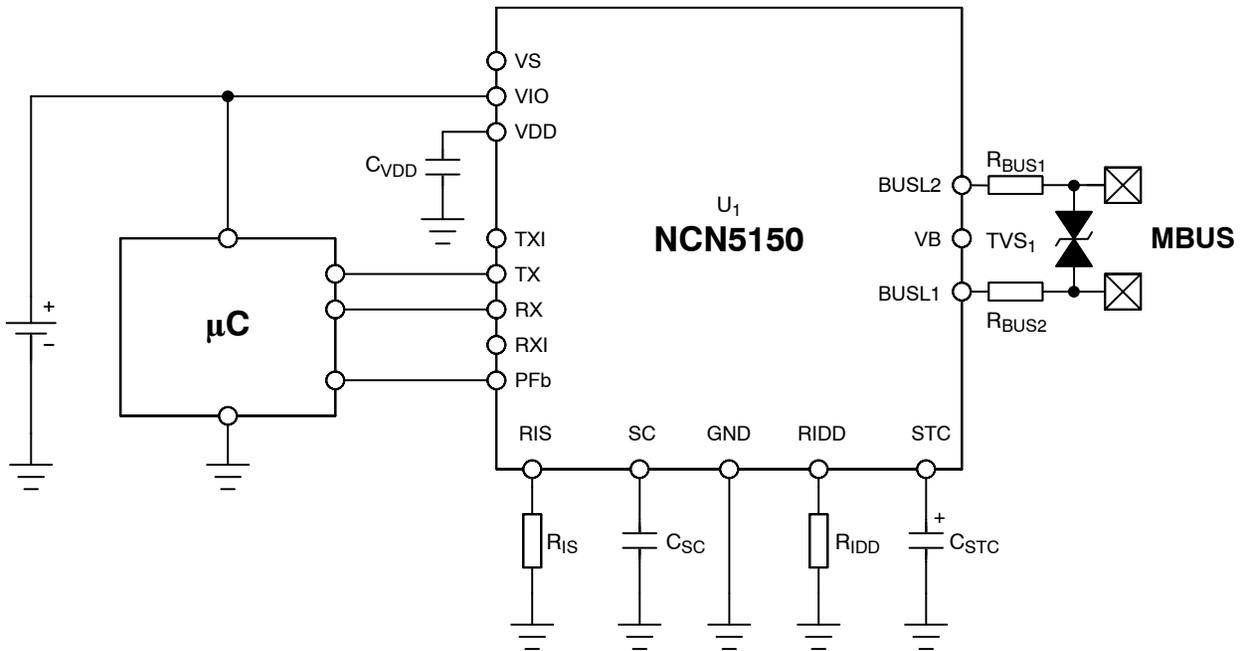
Figure 4. Application Schematic with External Power Supply (Battery)
