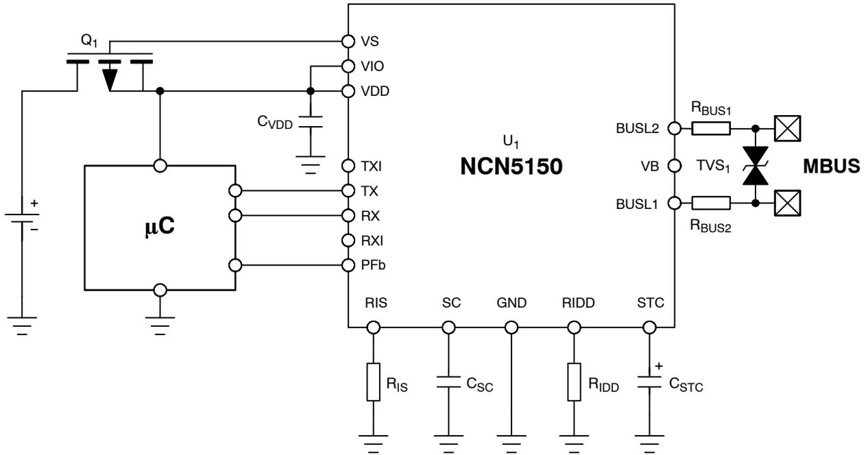
Figure 5. Application Schematic with Backup External Power Supply
