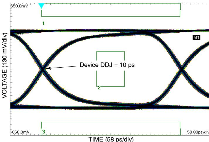
Figure 2. Typical Output Waveform at 2.488 Gb/s with PRBS 2<sup>23</sup>-1 (V<sub>INPP</sub> = 400 mV; Input Signal DDJ = 14 ps)
