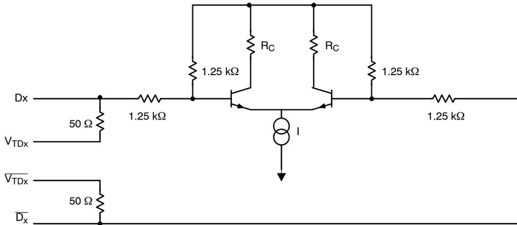
**Figure 10. Input Structure**
