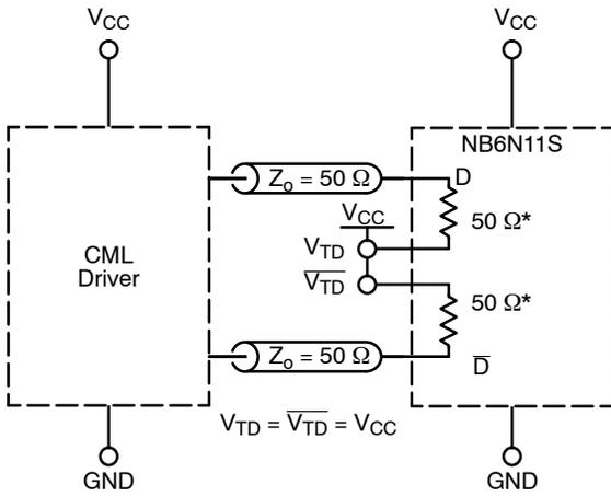
Figure 13. Standard 50  $\Omega$  Load CML Interface
