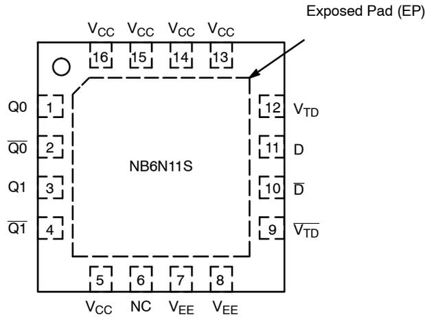
Figure 3. NB6N11S Pinout, 16-pin QFN (Top View)
