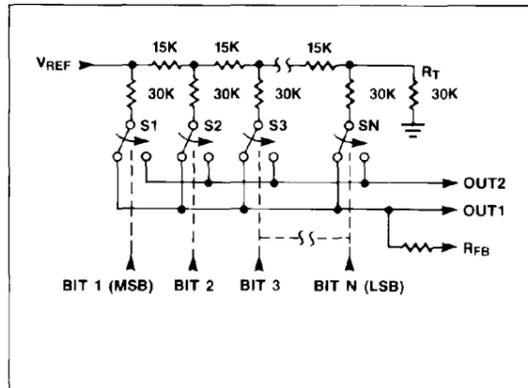
Figure 1. MX7543 Functional Diagram
