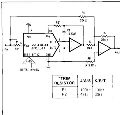
Figure 3. Bipolar Operation (4-Quadrant Multiplication)
