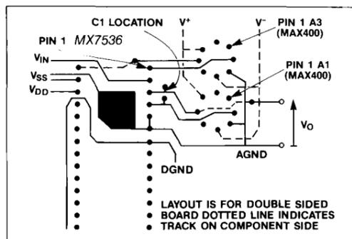
Figure 6. Suggested Layout for MX7536 Circuit of Figure 4
