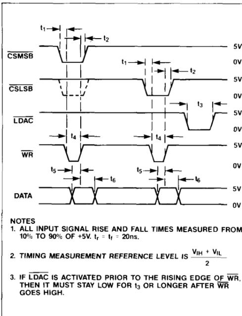
Figure 1. MX7536 Timing Diagram
