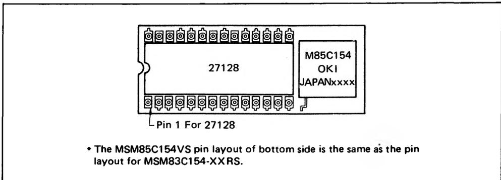
\* The MSM85C154VS pin layout of bottom side is the same as the pin layout for MSM83C154-XXRS.
