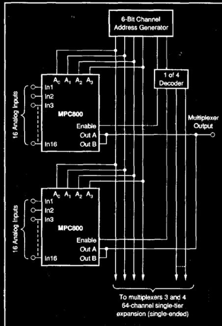
FIGURE 5. 32- to 64-Channel, Single-tier Expansion.
