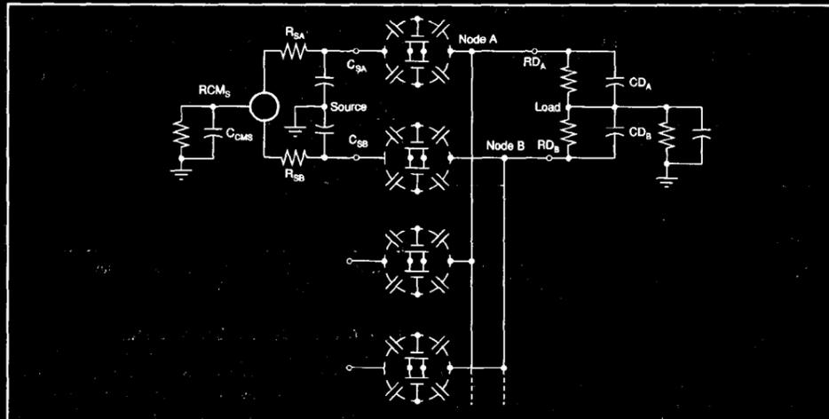
FIGURE 4. Settling and Common-Mode Effects (Differential).
