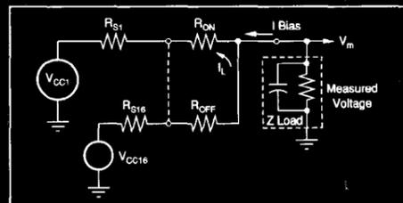
FIGURE 1. MPC800 Static Accuracy Equivalent Circuit (Single-ended Operation).
