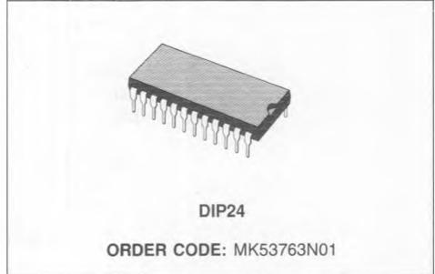
(DTMF) and PULSE (LD) modes of operation and it stores up to 13 18-digit numbers including the last number dialed. The user can store all 12 signalling digits plus access several unique functions with single key entries. These functions include : Last Number Dialed (LND), Softswitch, Flash, Pause and 12 memories (M1 - M9 and E1 - E3).
