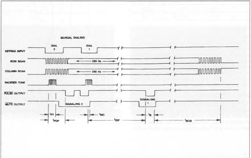
Figure 4B : MK5375 Timing Diagram – Tone Mode.
