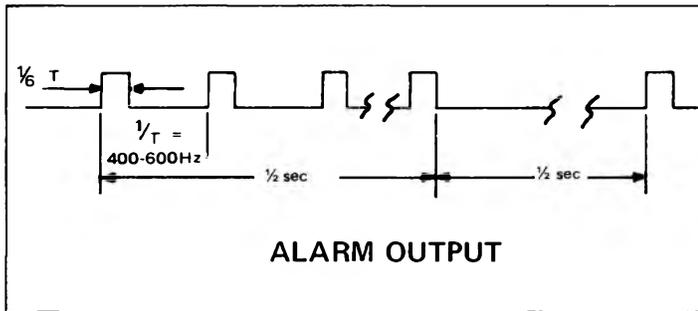
enabled and will activate 24 hours later at the alarm time. The output tone will be in the range of 400-600 Hz, and has a 1/6 duty cycle which conducts to  $V_{SS}$  50% of the time at a 1 Hz rate.
