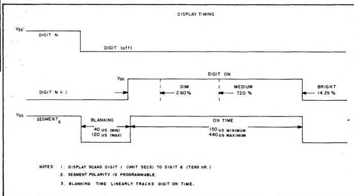
The Intensity Control Input provides the following degrees of display intensity:
