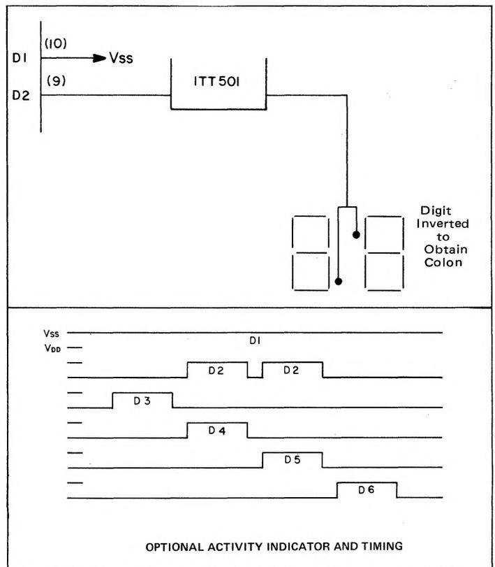
The AM/PM output operates with an 85% duty cycle at full intensity and conducts to  $V_{SS}$  for PM indication.
