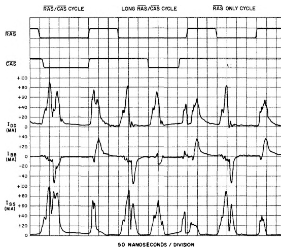
Fig. 5 Typical Current Waveforms
