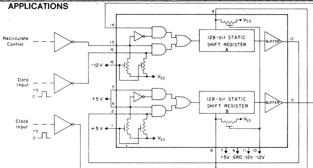
This shows the MK 1002 P connected to operate as a single, 256-bit, static shift register. Pull-up resistors are enabled at TTL driven inputs and disabled at MOS or DTL driven inputs. Any similar TTL/DTL device may be used in place of the inverters shown.
