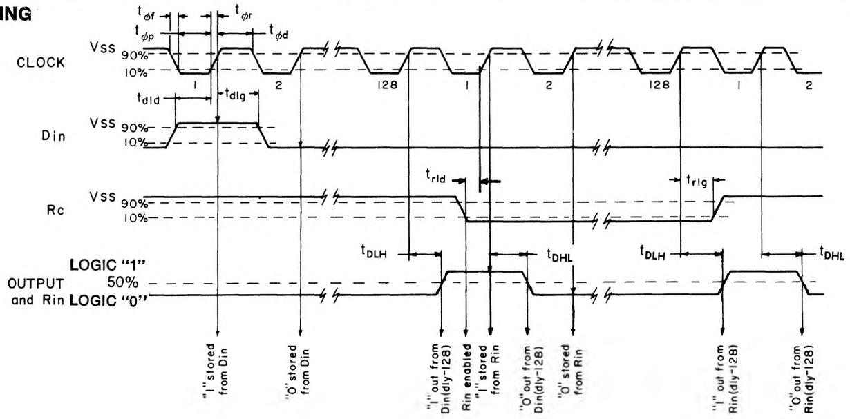
The timing diagram applies to either section of the dual shift register. The test conditions for these waveforms are illustrated below. A logic "1" is defined as +5V and a logic "0" is defined as 0V
