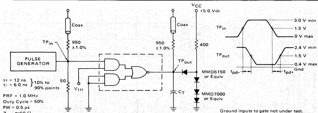
$C_T = 15 \text{ pF}$  = total parasitic capacitance, which includes probe, wiring, and load capacitances.
