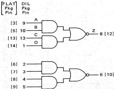
Positive Logic:  $Z = \overline{(A \bullet B)} + \overline{(C \bullet D)}$
