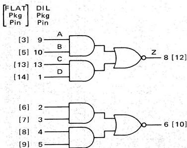
Positive Logic:  $Z = \overline{(A \cdot B)} + \overline{(C \cdot D)}$
