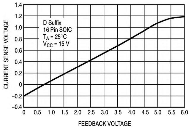
Figure 7. Feedback Voltage versus Current Sense Voltage
