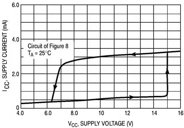
Figure 4. Supply Current versus Supply Voltage
