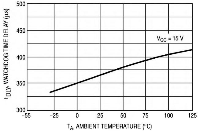
Figure 3. Watchdog Timer Delay versus Temperature
