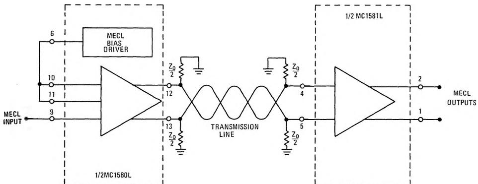
The output stage of the driver switches a current source between the two driver outputs in response to the input logic signals. Hence, a voltage differential that is a function of the line termination impedances is created on the twisted pair and at the input of the receiver. The receiver is designed to reject +3.5/-3.5 volts of common-mode voltage signals which may be present due to ground loop currents and noise coupled from nearby transmission lines.
