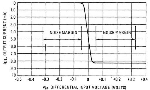
Hence the direct coupling of the driver and receiver to the line provides a built-in differential-mode noise immunity. The direct coupling also matches the line at all frequencies (often a problem with ac coupled lines). The recovery problem in ac coupling devices at high-signal repetition rates is also eliminated.
