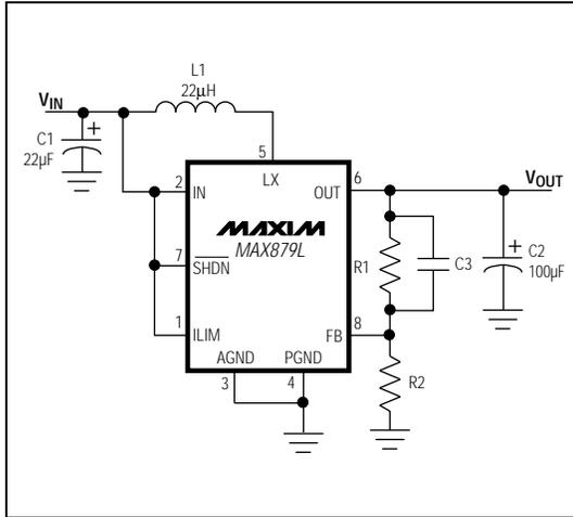
Figure 3. MAX879L Adjustable Voltage
