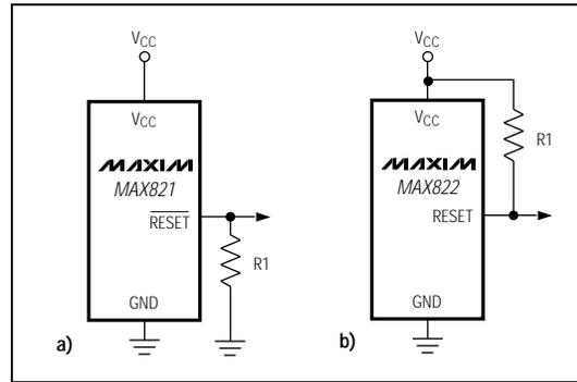
Figure 2.  $\overline{\text{RESET}}/\text{RESET}$  Valid to  $V_{CC} = \text{Ground}$  Circuit
