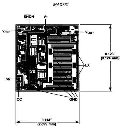
**NOTE:** CONNECT SUBSTRATE TO V+
