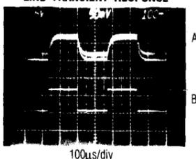
A:  $V_{OUT}$ , 50mV/div, DC-Coupled
