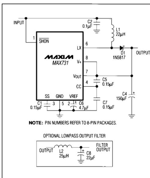
Figure 2a. MAX731 Standard Boost Application Circuit
