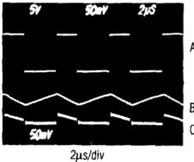
A: Switch Voltage (LX pin), 5V/div, 0V to +12.4V
