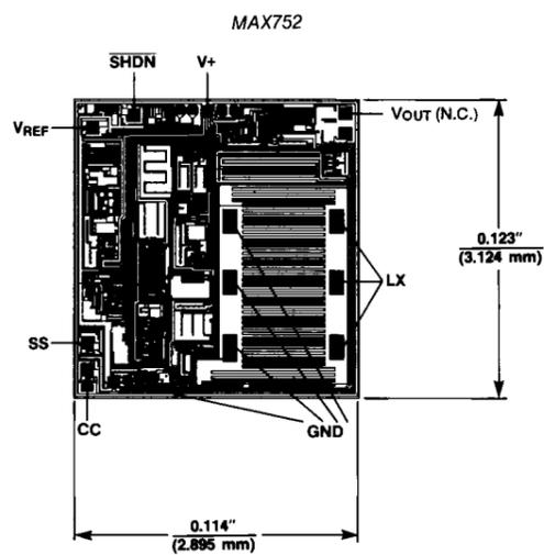
**NOTE:** CONNECT SUBSTRATE TO V+
