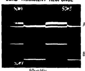
A:  $V_{OUT}$ , 50mV/div, DC-Coupled
