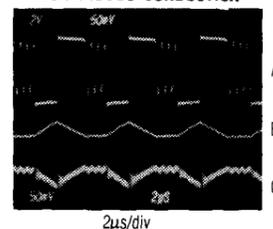
A: Switch Voltage (LX pin), 2V/div, 0V to +5V
