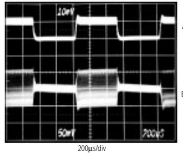
A:  $I_{LOAD} = 0\text{mA to } 200\text{mA}$
