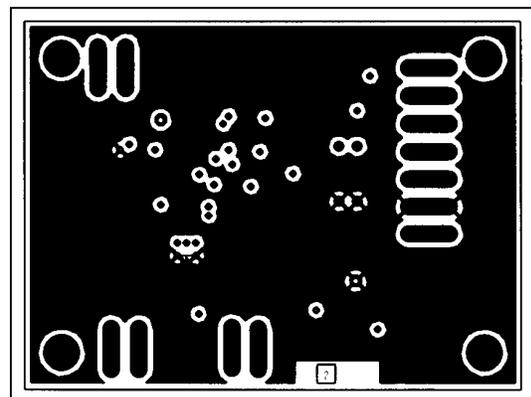
Figure 6. MAX624 PC Board Layout—VSWITCHED Plane
