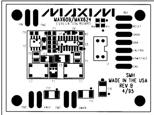
Figure 3. MAX624 PC Board Component Placement Guide
