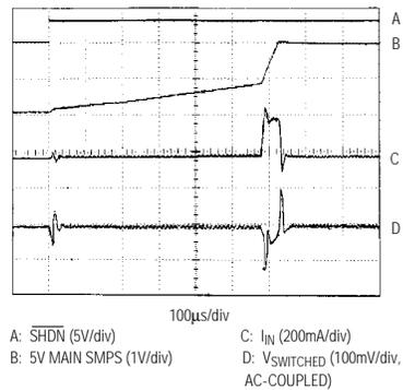
**START-UP INRUSH CURRENT ( $V_{IN} = 3.3\text{V}$ )**
