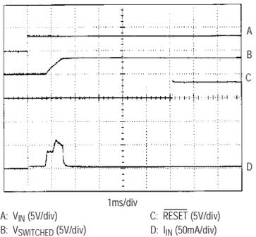
**START-UP INRUSH CURRENT ( $V_{IN} = 5\text{V}$ )**
