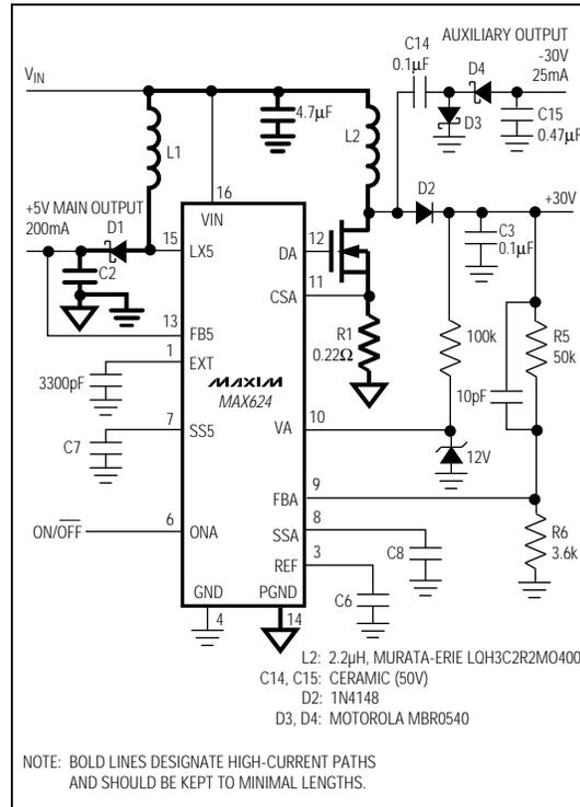
Figure 11. Negative 30V Auxiliary Output Application Circuit
