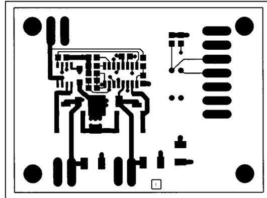
Figure 5. MAX624 PC Board Layout—Component Side
