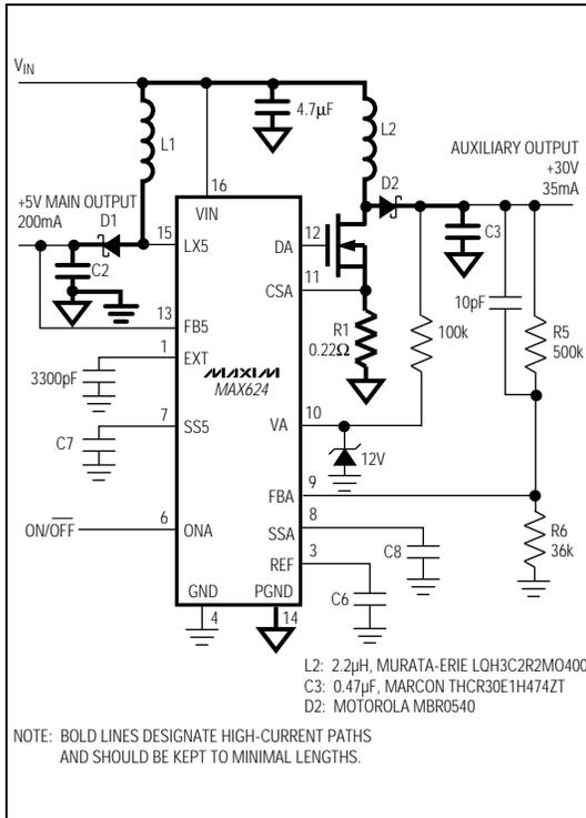
Figure 10. Positive 30V (35mA) Auxiliary Output Application Circuit
