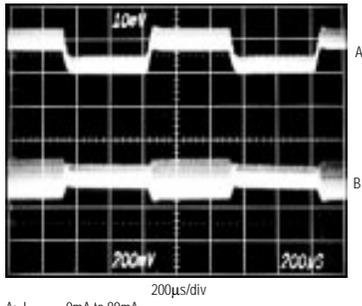
A:  $I_{LOAD} = 0\text{mA to } 80\text{mA}$
