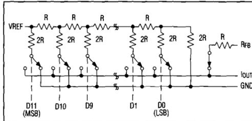
Figure 1. MAX543 Simplified Circuit
