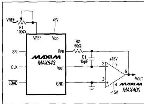
Figure 3. Unipolar Operation
