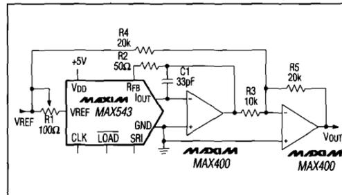
Figure 4. Bipolar Operation
