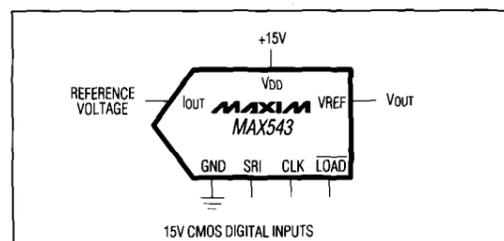
Figure 5. Single-Supply Operation Using Voltage-Switching Mode
