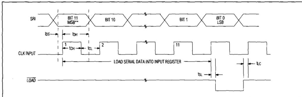
Figure 2. Write-Cycle Timing Diagram
