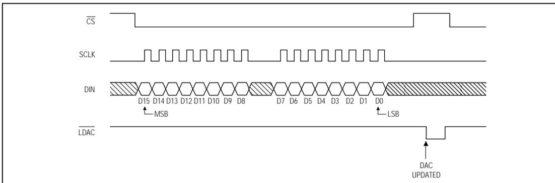
Figure 3b. 4-Wire Interface Timing Diagram
