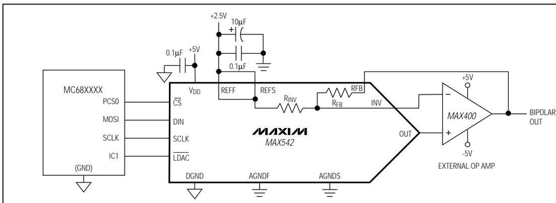
Figure 2b. Typical Operating Circuit—Bipolar Output
