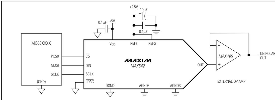
Figure 2a. Typical Operating Circuit—Unipolar Output
