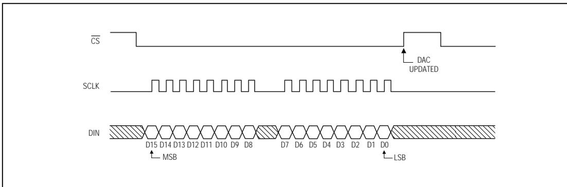
Figure 3a. 3-Wire Interface Timing Diagram ( $\overline{LDAC} = \text{DGND}$ )
