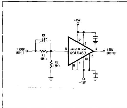
Figure 5. High Speed High Voltage Attenuator
