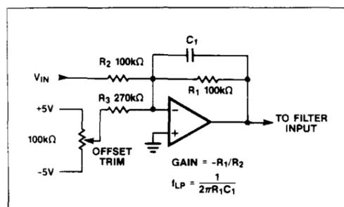
Figure 18. Circuit for DC Offset Adjustment
