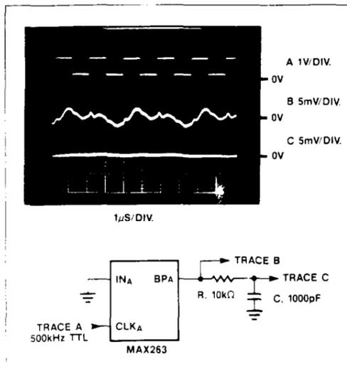
Figure 15. MAX263 Bandpass Output Clock Noise
