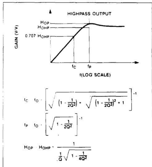
Figure 11. Second-Order Highpass Characteristics
