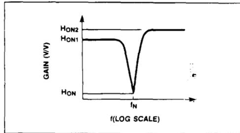
Figure 12. Second-Order Notch Characteristics
