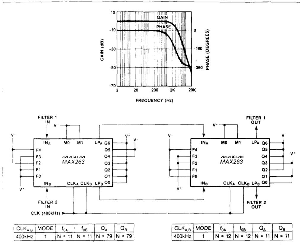
Figure 21. Dual Tracking 3kHz 4th-Order Lowpass
