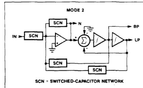
Figure 5. Filter Mode 2: Second-Order Bandpass, Lowpass and Notch
