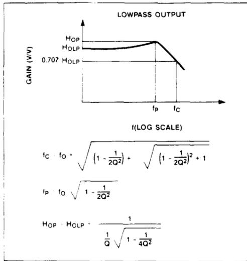
Figure 10. Second-Order Lowpass Characteristics
