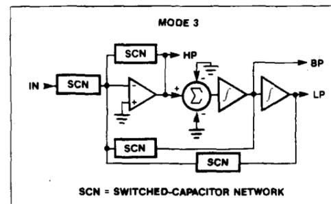
Figure 6. Filter Mode 3: Second-Order Bandpass, Lowpass and Highpass
