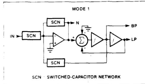
Figure 4. Filter Mode 1: Second-Order Bandpass, Lowpass and Notch
