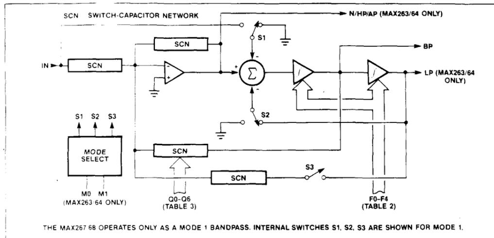
Figure 1. Filter Block Diagram (One Second-Order Section)
