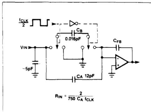
Figure 16. MAX263/64/67/68 Input Model
