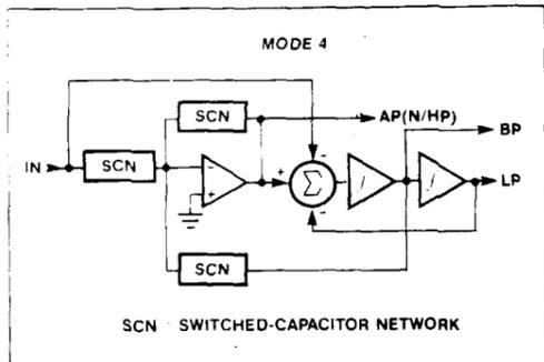
Figure 8. Filter Mode 4: Second-Order Bandpass, Lowpass and Allpass
