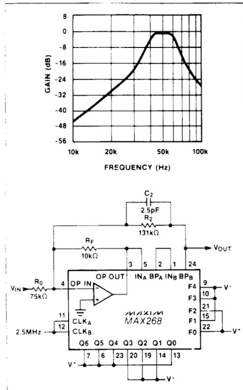
Figure 19. 4th-Order 50kHz Chebyshev Bandpass Using Multiple Feedback
