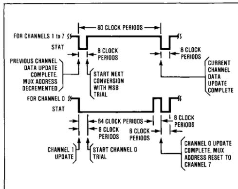
Figure 2. STAT Timing Diagram
