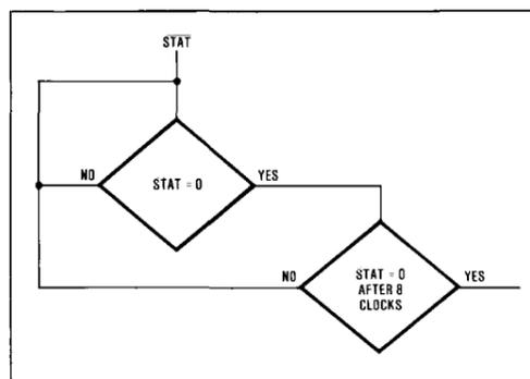
Figure 4. Software Channel Identification
