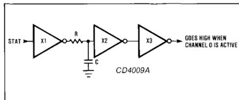
Figure 3. Hardware Channel Identification
