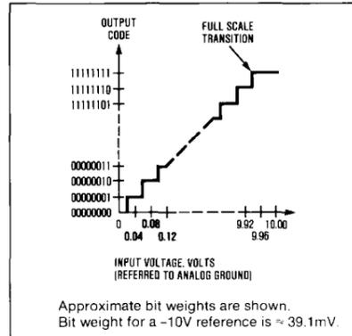
Figure 6. Unipolar (0 to +10V) Transfer Characteristic
