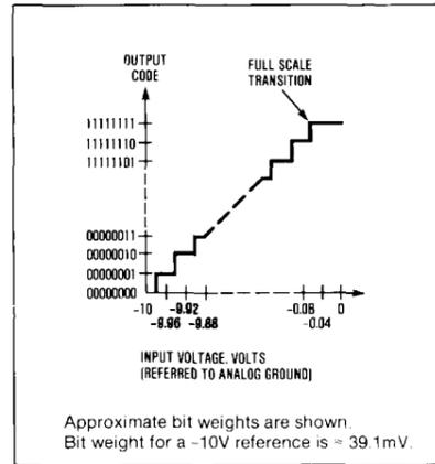
Figure 8. Unipolar (0 to -10V) Transfer Characteristic
