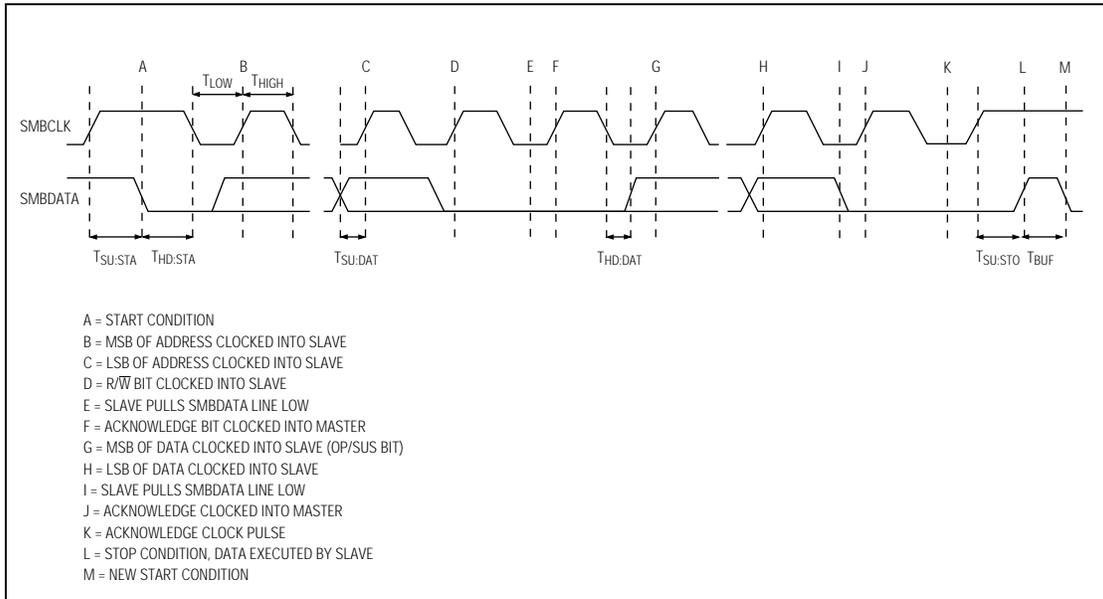
Figure 2. SMBus Write Timing Diagram
