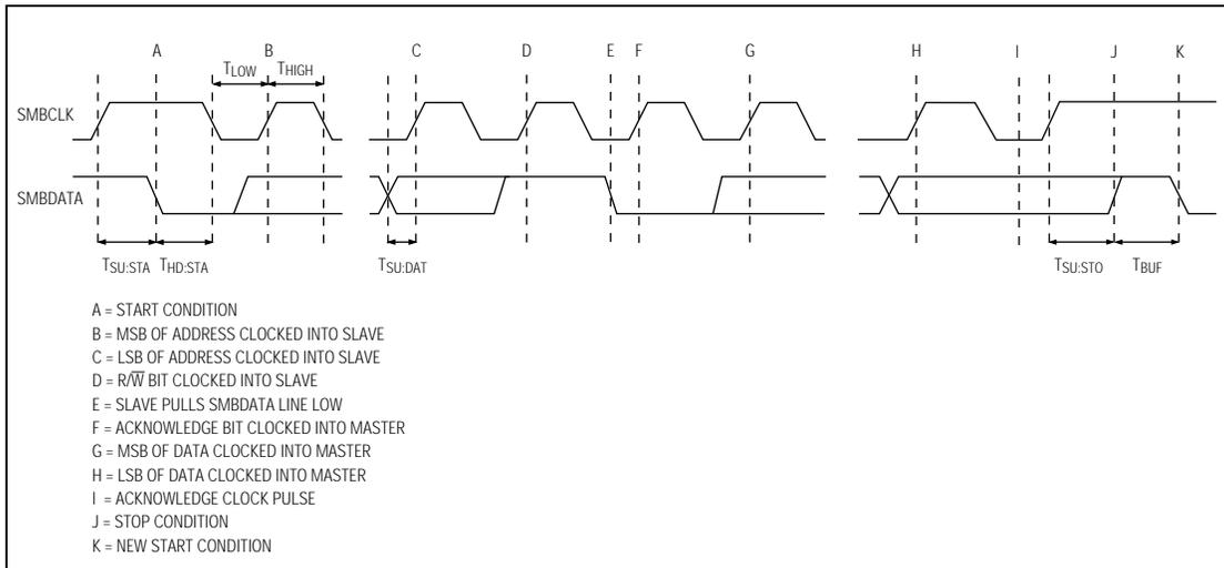
Figure 3. SMBus Read Timing Diagram
