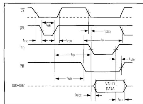
Figure 5. WR-RD Mode Timing ( $t_{RD} > t_{INTL}$ ).
