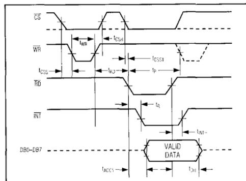
Figure 6. WR-RD Mode Timing ( $t_{RD} < t_{INTL}$ ).
