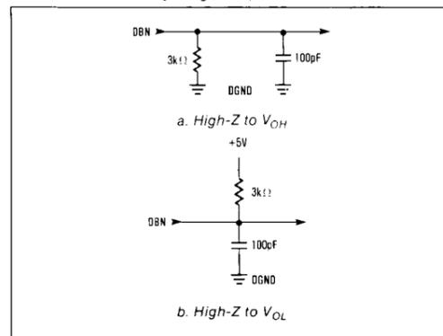
Figure 1. Load Circuits for Data Access Time Test
