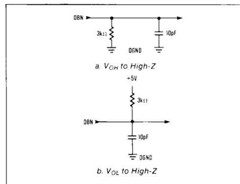
Figure 2. Load Circuits for Data Hold Time Test
