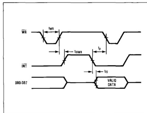
Figure 8. WR-RD Mode Stand-Alone Timing  $\overline{CS} = \overline{RD} = 0$ .
