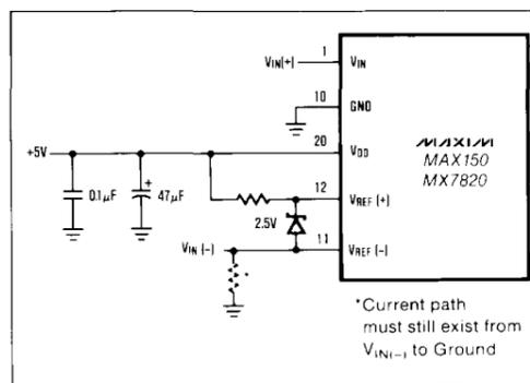
Figure 10d. Input Not Referenced to GND.
