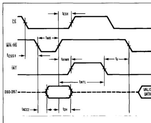
Figure 7. WR-RD Mode Pipe-Lined Timing  $WR = RD$ .
